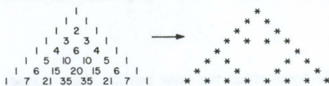
Figure 4. An algebraic construction for the configurations of a cellular automaton starting from a state containing a single site with value 1 and evolving according to the modulo-two rule 90. The rule is illustrated in Fig. 1, and takes the value of a particular site to be the sum modulo two of the values of its two neighboring sites at the previous time step. The value of a site at a given time step is then just the value modulo two of the corresponding binomial coefficient in Pascal’s triangle.
