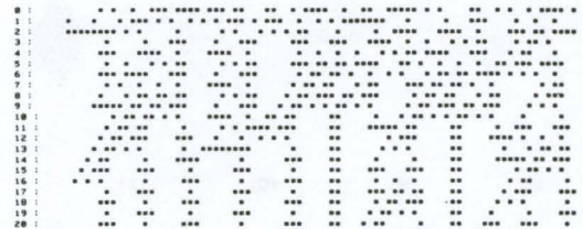
Figure 31. Evolution of two typical one-dimensional cellular automata with two states per site in which the value of a site at a particular time step is determined by the preceding values of a neighborhood of five sites containing the site, its nearest neighbors, and its next-nearest neighbors. The initial configurations in the lower row are typical of disordered configurations, in which each site has value one with probability \frac{1}{2} .
