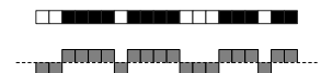
A sequence of discrete elements and a possible corresponding waveform for a sound.
